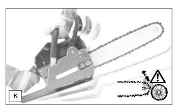
The MAKITA models comes with an inertia chain brake as standard equipment. If kickback occurs due to contact of the guide-bar tip with wood (see SAFETY PRECAUTIONS), the chain brake will stop the chain through inertia if the kickback is sufficiently strong. The chain will stop within a fraction of a second.
